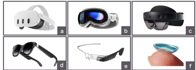
Figure 3: Typical form factors of CR devices: (a) a headset with no eye contact, e.g., Meta Quest 3; (b) a headset with simulated social cues, e.g., Apple Vision Pro; (c) a headset with transparent lenses, e.g., Microsoft HoloLens; (d) sunglasses, e.g., Nreal Air; (e) glasses, e.g., Google Glass; (f) contact lenses.
