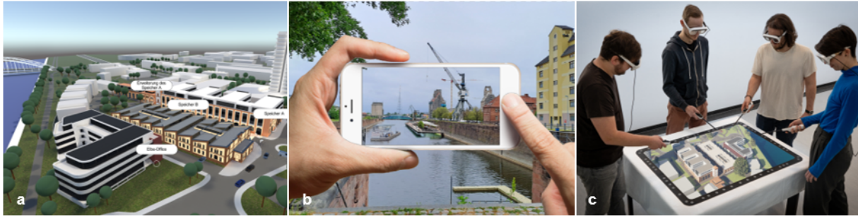
Figure 1: Early prototyping stage of the urban cross-reality environment. a) Bird's eye view of a section of the virtual model as it would be seen in the current web interface prototype. b) Illustration of mobile AR-overlaid content (the waterside café and the raft are virtual) in the post-industrial environment. c) Collaborative HMD-based interaction with the environment model. The prototype in the image is implemented with the Tilt Five augmented reality device (Tilt Five Inc., Fremont, CA, USA).
