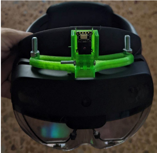
Figure 1: 3D printed case housing FLIR Lepton 3.5 on Hololens 2
