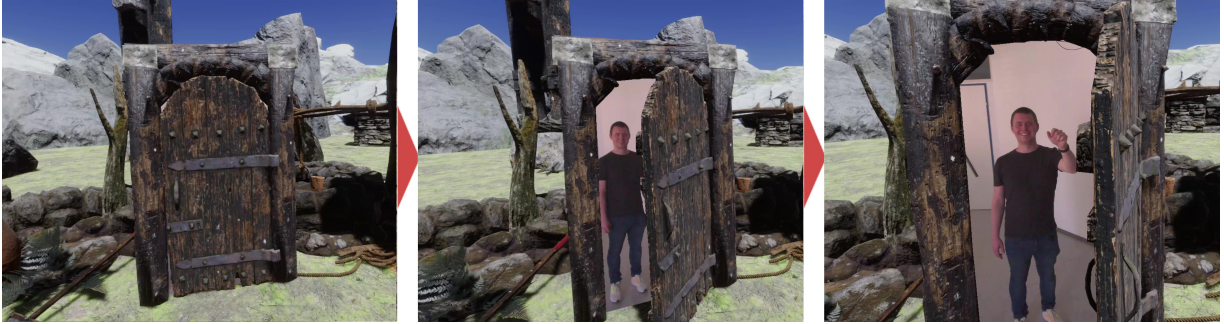
Figure 1: An early prototype shows how the Door metaphor could be designed and implemented. The virtual door appears in the virtual environment at the position of the incoming bystander. When the door opens, it activates a video-based pass-through mode, allowing the HMD user to visually perceive the real environment beyond the virtual door.
