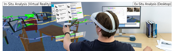
Figure 1: RELIVE [15] is a CR application that combines an immersive analytics virtual reality view (left) with a synchronized visual analytics desktop view (right). The application state of RELIVE is kept in sync between both views using Colibri.
